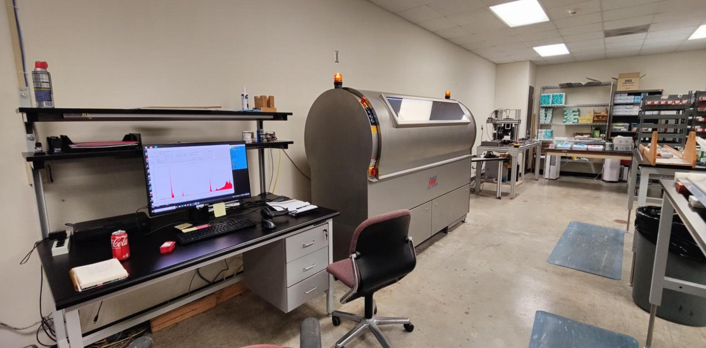
X-Ray Fluorescence Scanner at the College Station Core Repository
