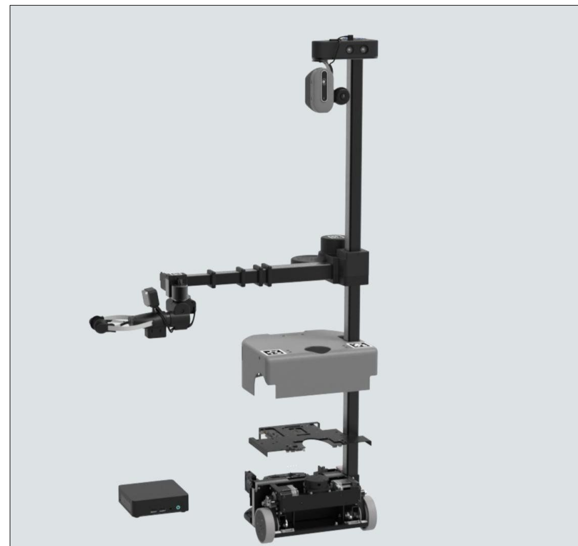
Figure 1: Visual depiction of the Stretch 3 robot
